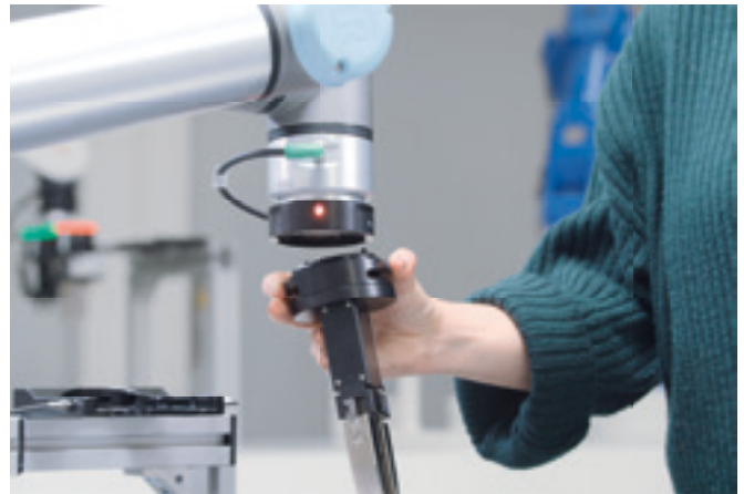
Manual exchange with one-hand function within seconds.
