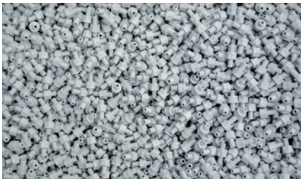
Large-scale series production of plastic parts made of POM
