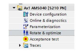
The One Button Turning function is used to optimize control parameters.
