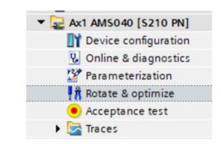
The One Button Turning function is used to optimize control parameters.
